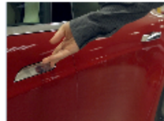
Driver's door handle is stuck.
