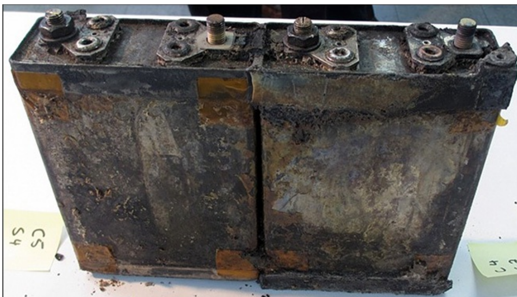
THIS IS AN ACTUAL BOEING BATTERY AFTER AN IN-FLIGHT FIRE
