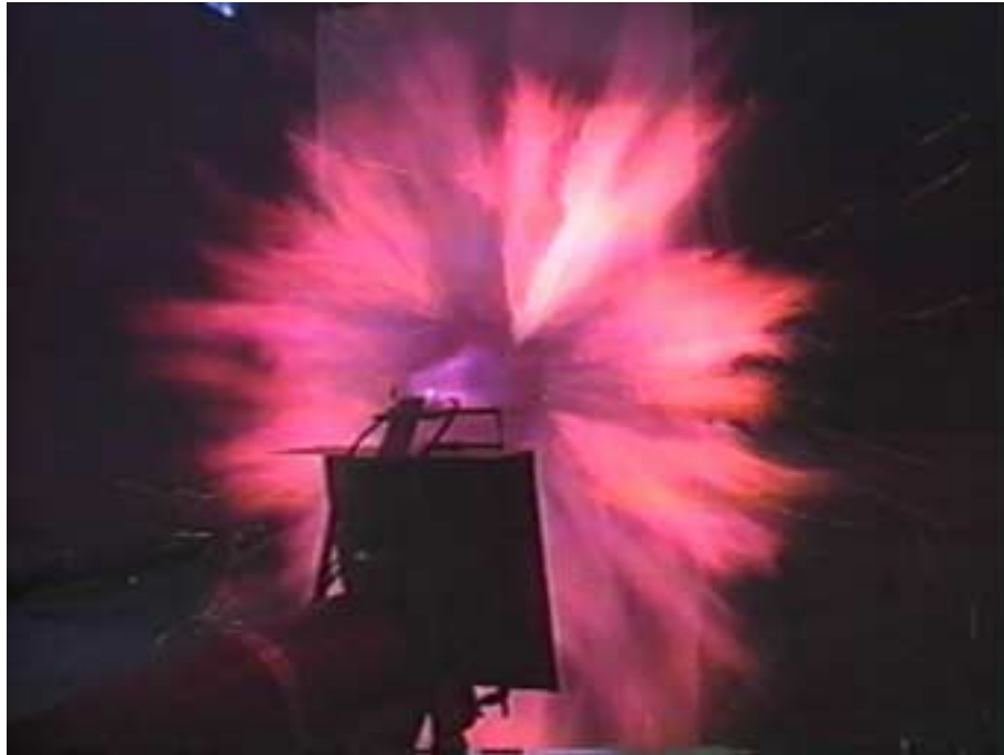
Figure C 9 - Hydrogen flame impingement, early in burn
