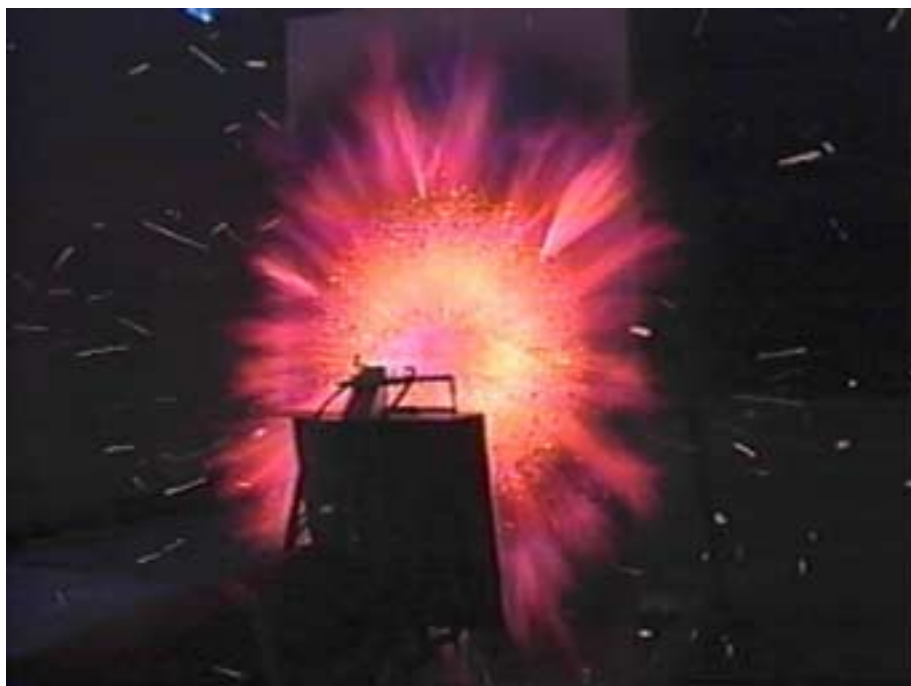
Figure C 10 - Hydrogen flame impingement on gypsum wallboard (paper cover burning)
