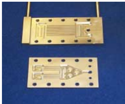
Figure 6. Catalytic reactor (top) and fuel mixer components (bottom).
