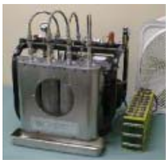
Figure 2: Left: Ovonic Hydrogen ICE Generator. Right: Ovonic Metal Hydride Storage system integrated with a 2.8 KWe PEM Fuel Cell. Hydrogen stored provides 3 hours of back-up power at 2KWe.
