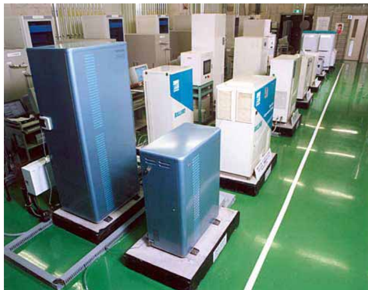
Range of residential systems being tested by the Japan Gas Association (Source: Japan Gas Association)
