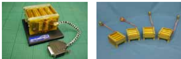
Figure 12 Eight-cell Battery Building Block
