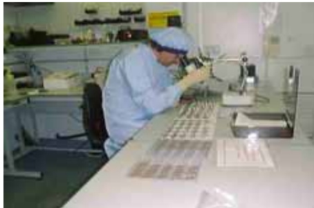
Figure 4 Cell Destructive Physical Analysis
