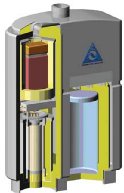
Ceramic Fuel Cells has patented Solid Oxide Fuel Cell Technology that can be incorporated into this small Combined Heat and Power (CHP) unit. It will generate power and provide hot water service for homes.
