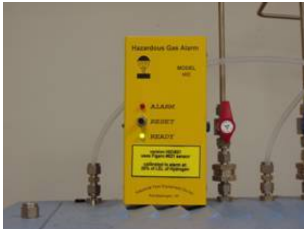
PEM Fuel Cell Dual Station with a Hydrogen Sensor
