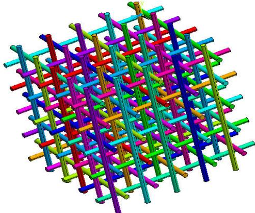
Conformable pressure vessels efficiently use available space in the vehicle, increasing truck hydrogen delivery capacity
