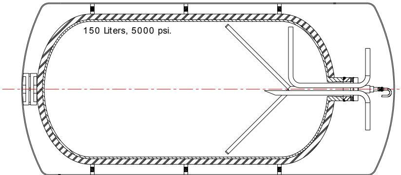
Cryo-compressed hydrogen (~80 K, ~5000 psi) requires considerably less storage energy (~18% of LHV) than LH<sub>2</sub> (~35% of LHV), has high density (~63 kg/m<sup>3</sup>), and considerably lower evaporative losses than LH<sub>2</sub>.
