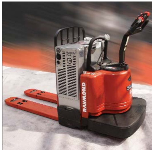
Raymond has been testing numerous fuel cell powered vehicles such as this pallet truck
