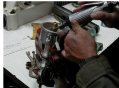
Figure 14 - Grinding out 7 of the 8 vanes.
