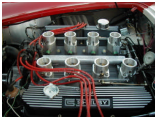
Figure 16 – View of Engine Converted to Run on Hydrogen
