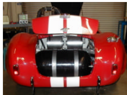
Figure 7 – Hydrogen storage tank
