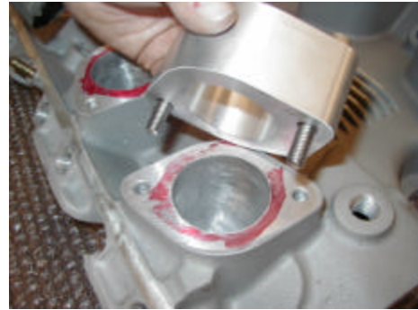
Figure 6 – Match porting injector with intake manifold
