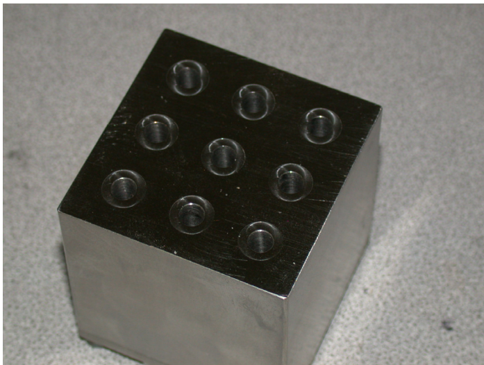
Image of a 3x3 micro-reactor arrays
