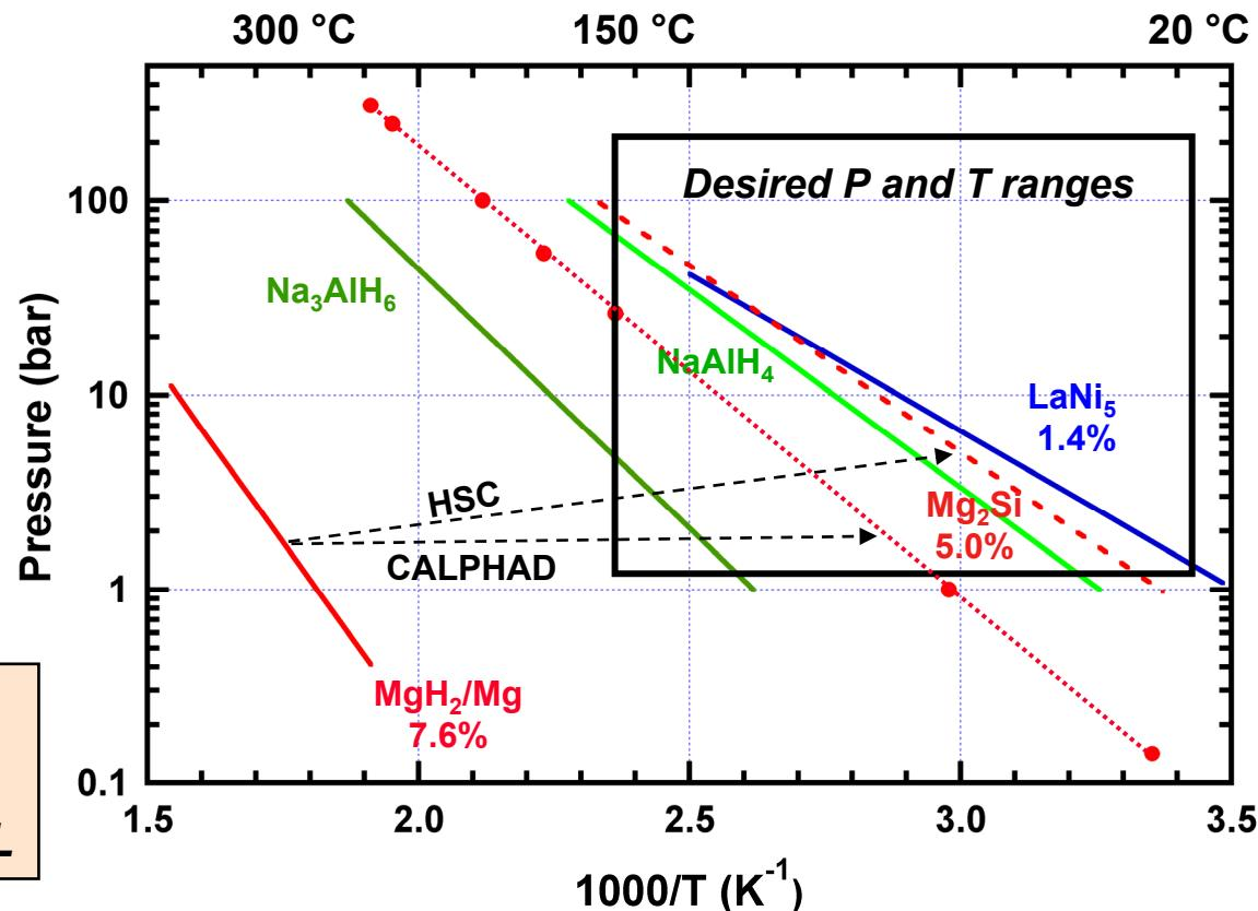
Equilibrium conditions predicted by thermodynamic modeling software (HSC and CALPHAD) for  $\text{MgH}_2/\text{Si}$  system in desired temperature and pressure range
