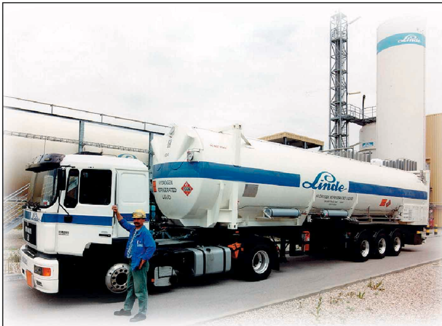
Figure 3. Trailer for LH 2 transport (total weight, 40 tons; hydrogen load, 3370 kg). Compare this with the trailer for CGH 2 shown in Figure 1 of the article by Irani in this issue (total weight 40 tons; hydrogen load, 530 kg at 20 MPa). The LH 2 trailer is able to transport more than six times the hydrogen load of the CGH 2 trailer.
