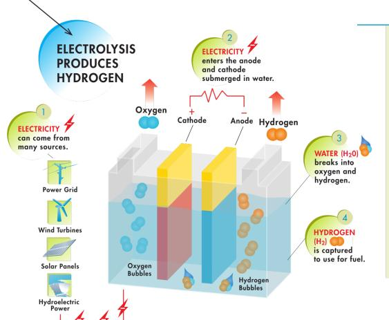
Electrolysis passes a current through water, splitting the water molecules into hydrogen and oxygen. The electrolyzer contains a thin membrane coated with a catalyst to speed the reaction. The hydrogen is stored for fuel and the oxygen is released into the atmosphere.
