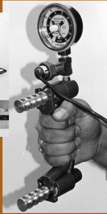
Photo 1 (far left): Experimental handle configured as a screwdriver. One handle segment is removed to reveal the instrumented core. Photo 2 (left): Hand dynamometer. A pressure transducer was inserted between the dynamometer body and dial gauge.
