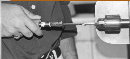
Photo 1 (far left): Experimental handle configured as a screwdriver. One handle segment is removed to reveal the instrumented core. Photo 2 (left): Hand dynamometer. A pressure transducer was inserted between the dynamometer body and dial gauge.
